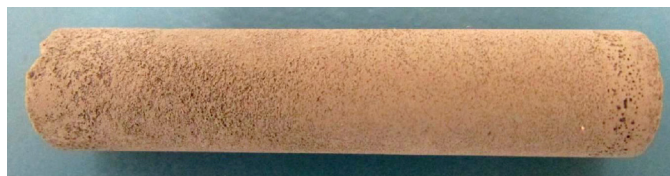
Sintered catalyst cylinder developed for Umpqua Research's Continuous Bosch Reactor.
