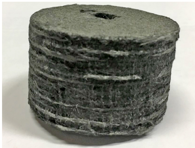
Substrate loaded with carbon from Honeywell Aerospace's Carbon Vapor Deposition process.
