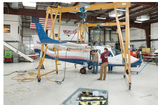
Wing Installation at Scaled Composites
