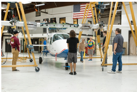
Wing Installation at Scaled Composites
