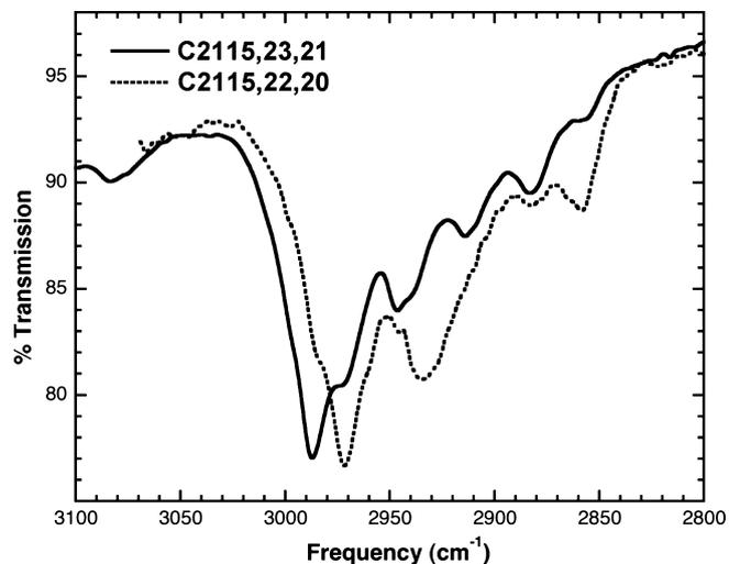
Fig. 2. Infrared spectra in the C-H stretching region taken approximately  $560\ \mu\text{m}$  away from the centers of tracks C2115,22,20 (dashed line) and C2115,23,21 (solid line) in their respective keystones.
