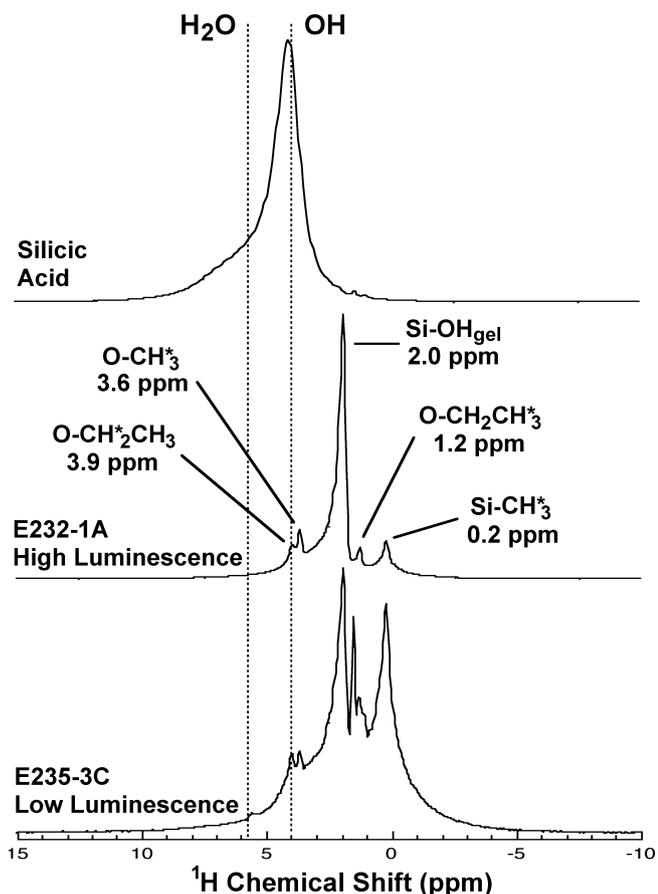
Fig. 5.  $^1\text{H}$  solid state NMR spectra of silicic acid (top) and aerogel samples E232-1A (middle) and E235-3C (bottom). In addition to Si-OH and structural (nonliquid) water that contributes to the very broad peak spanning the entire frequency range, the aerogel samples reveal sharp peaks that indicate the presence of hydrogen in silicate ethoxide and methoxide functional groups, as well as silicone methyl groups.
