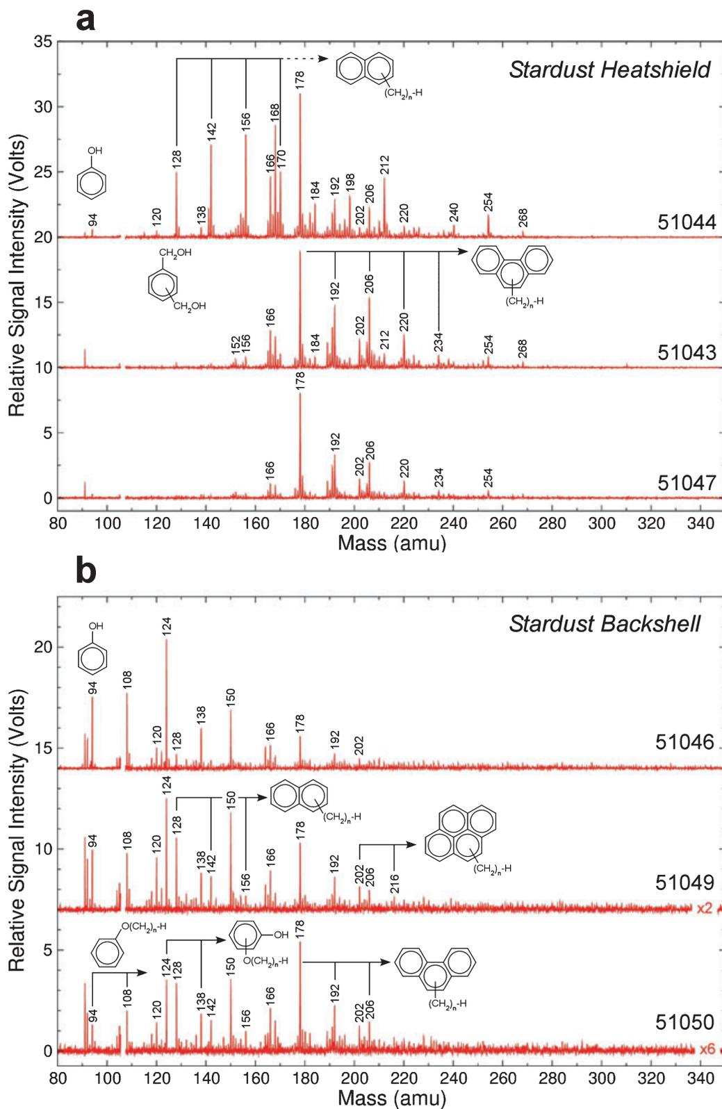
Fig. 15. Mass spectra taken from samples from SRC locations on the a) heatshield and b) backshell as noted in Fig. 14. Species detected include 1–4 ring aromatic species, their  $C_n$ -alkylated homologues, oxygenated aromatics, and low mass phenolic aromatics. The abundance and distribution of these organic species varies significantly between samples, but the distributions do not match those of aromatic species found within aerogel impact tracks in the Stardust collector (see text).
