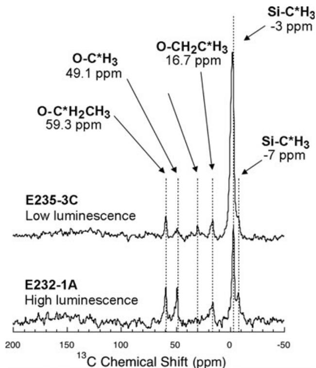
Fig. 4. <sup>1</sup>H-<sup>13</sup>C cross polarization solid state NMR spectra of aerogel samples from tiles E235-3C (low luminescence) and E232-1A (high luminescence). The presence of carbon corresponding to silicate bound ethoxide and methoxide, along with a more abundant methyl silicone moiety at approximately -3 and -7 ppm, is clearly revealed.
