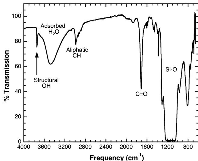
Fig. 1. Infrared spectrum of an approximately  $10\ \mu\text{m} \times 10\ \mu\text{m}$  spot on C2115,23,21, a keystone extracted from the C2115 Stardust aerogel flight cell. The strong Si-O, C=O, aliphatic  $-\text{CH}_2-$  and  $-\text{CH}_3$ , structural  $-\text{OH}$ , and adsorbed  $\text{H}_2\text{O}$  absorption features were seen at all the spots examined and their presence is typical of Stardust flight aerogels.
