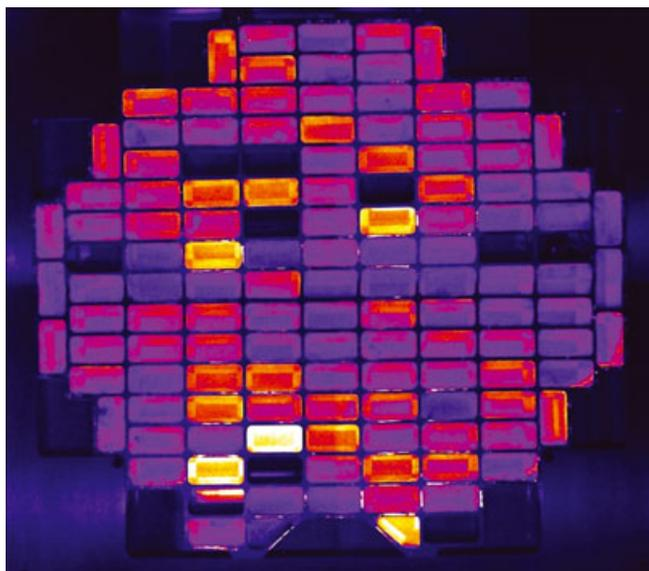
Fig. 7. Photograph of the tile luminescence in the cometary tray. Dark rectangles represent locations where tiles had already been removed for PE analysis. It is clear from these images that the luminescence is not uniformly or smoothly spread across the collector tray.
