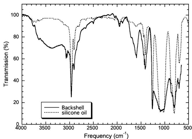
Fig. 13. The 4000–650  $\text{cm}^{-1}$  (2.5–15.4  $\mu\text{m}$ ) IR spectra of backshell SLA sample E51049 (solid line) compared with the Omnic® library database spectrum of silicone oil (dashed line). The similarities in the spectra are consistent with the presence of Si-bearing organics in both materials.
