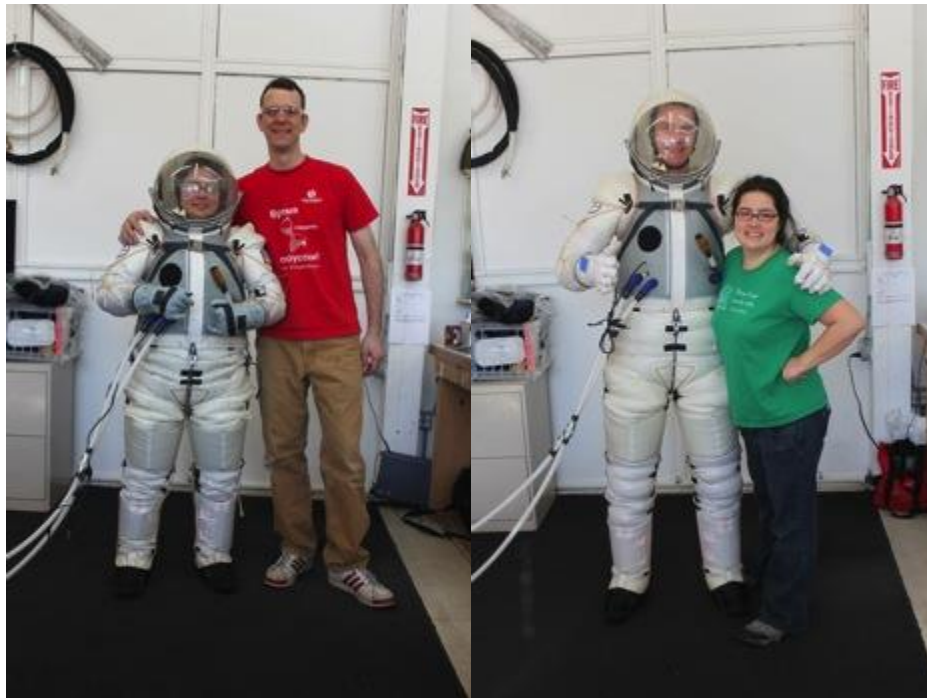
Figure 1. FFD's IVA Space Suit, +3 PSIG, Illustrating a 14" vertical adjustment range
