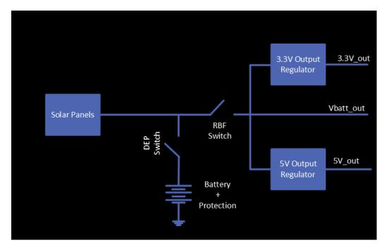
Power system design used successfully in multiple flight projects
