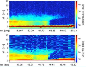
Jan. 2019 – Near-collocated measurements of vertical rain reflectivity profiles from RainCube (top) and GPM's Ka-band radar (bottom) RainCube points Nadir while GPM scans along-track
