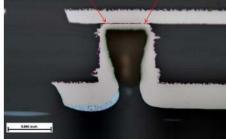
PCB manufacture passed vendor QA, but NASA detected open circuits
