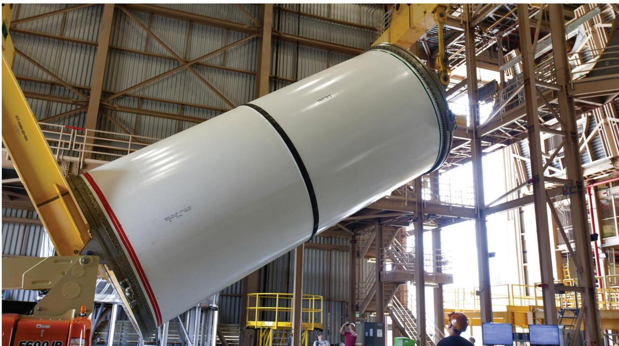
Technicians watch as a crane and special mechanism begin breaker, or flipping, of the mated Thrust Resistance Structure and Guidance Control Assembly for the Orion Program's Ascent Abort-2 flight test during practice, or pathfinder activities, June 22, 2018, inside the Rotation, Processing and Surge Facility at NASA's Kennedy Space Center in Florida. Photo credit: NASA/Ben Smegelsky
