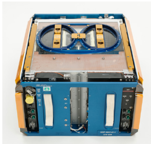
Rodent Transporter - for transportation to and from the International Space Station. Image credit: NASA / Dominic Hart
