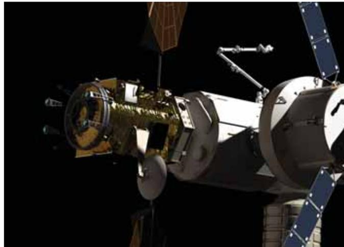
*Power and Propulsion Element (PPE) with Hall thruster electric propulsion systems.*
