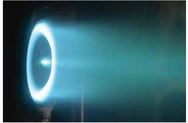
*Hall Effect Rocket with Magnetic Shielding (HERMeS) Technology Development Unit shown during testing in Vacuum Facility-5 at NASA Glenn Research Center.*
