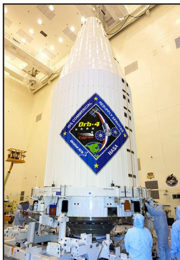
Engineers encapsulate the Orbital ATK enhanced Cygnus spacecraft in a protective payload fairing inside the Payload Hazardous Servicing Facility at NASA's Kennedy Space Center in Florida. Photo credit: United Launch Alliance
