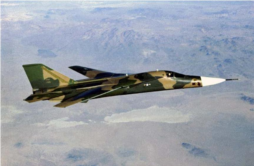
**Figure 5-2.** NASA, the Air Force, Boeing, Honeywell, and Pratt & Whitney used the prototype F-111E for integrated propulsion control system (IPCS) flights from 1975 to 1976. (NASA)
