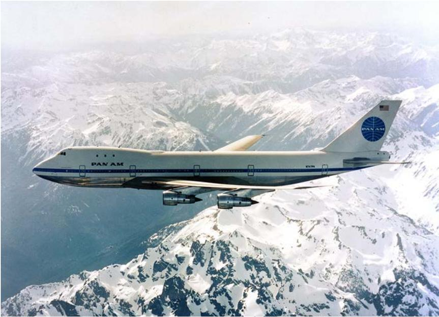
Figure 4-3. The high-bypass Pratt & Whitney JT9D powered a new generation of airliners, including the Boeing 747 jumbo jet. (NASA)
