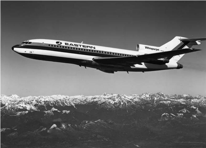
**Figure 4-2.** The Boeing 727 featured three Pratt & Whitney JT8D turbofans. (Boeing)
