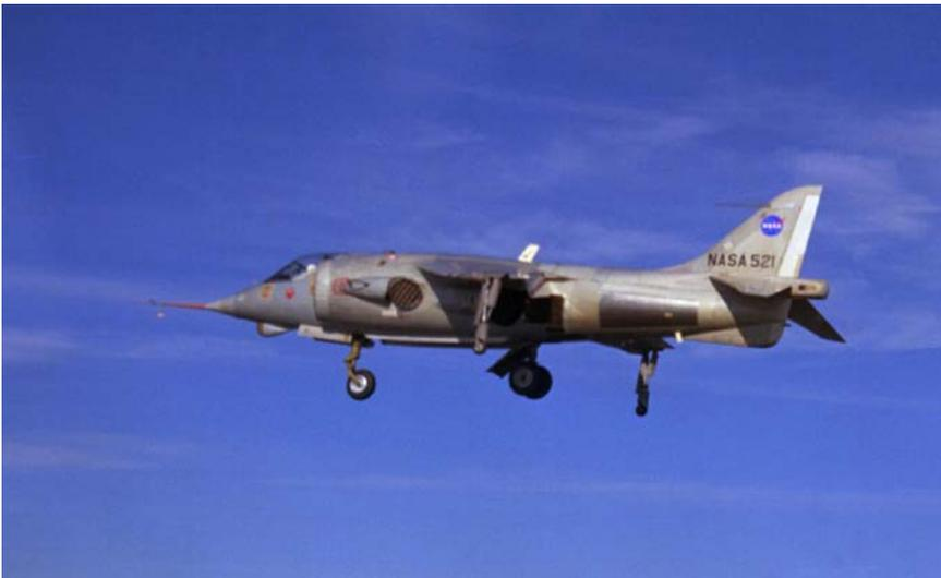
**Figure 3-2.** The Kestrel V/STOL research aircraft. (NASA)
