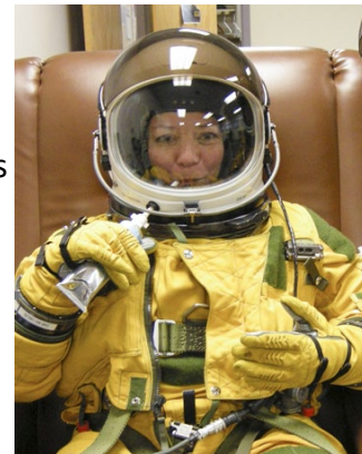
Air Force U-2 suits have a port for food and pills in the hard shell.
