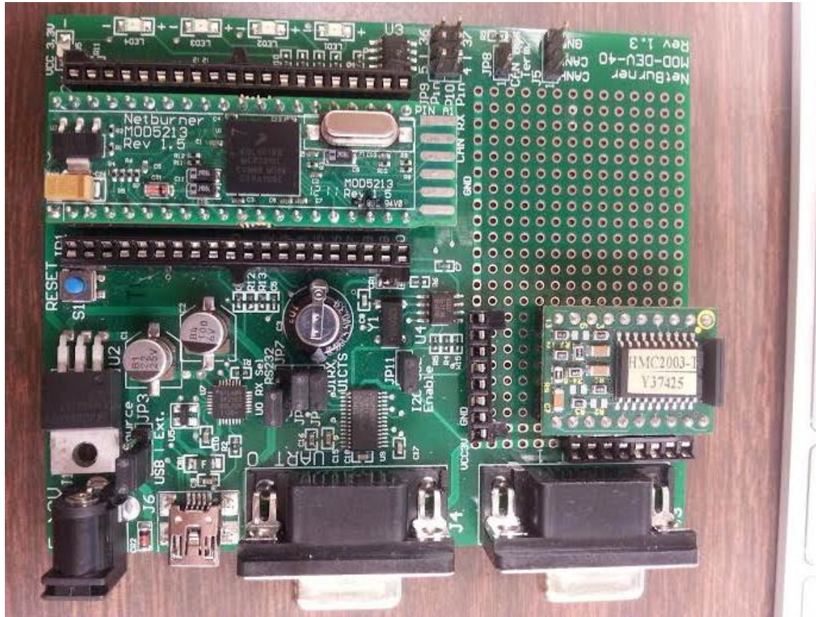
Netburner micro controller connected to the MOD-DEV-40 development board along with HMC2003 Magnetometer
