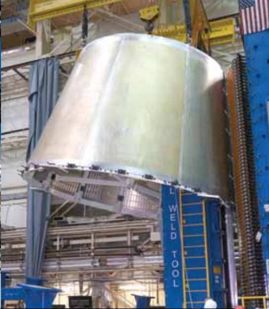
SLS LAUNCH VEHICLE STAGE ADAPTER CONE NASA Marshall Space Flight Center, Alabama
