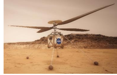
Figure 13. Ingenuity has long rotor blades because of the thin Martian atmosphere. Credit: NASA
