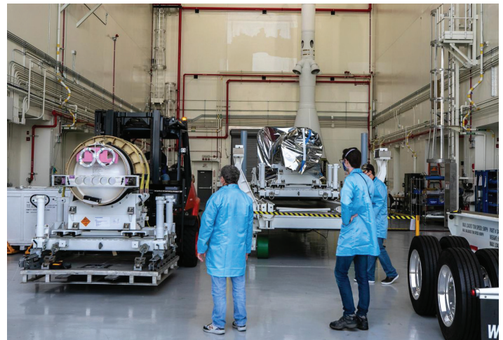
The last of three motors required to assemble the Launch Abort System (LAS) for NASA's Artemis II mission, the attitude control motor (ACM), arrived at Kennedy Space Center on Aug. 28, 2020, and was delivered to the Launch Abort System Facility. During launch of Orion atop the agency's Space Launch System rocket, the LAS motors work together to separate the spacecraft from the rocket in the unlikely event of an emergency during launch. The ACM operates to keep Orion's crew module on a controlled flight path in the event it needs to jettison and steer away from the rocket. Photo credit: NASA/Ben Smegelsky
