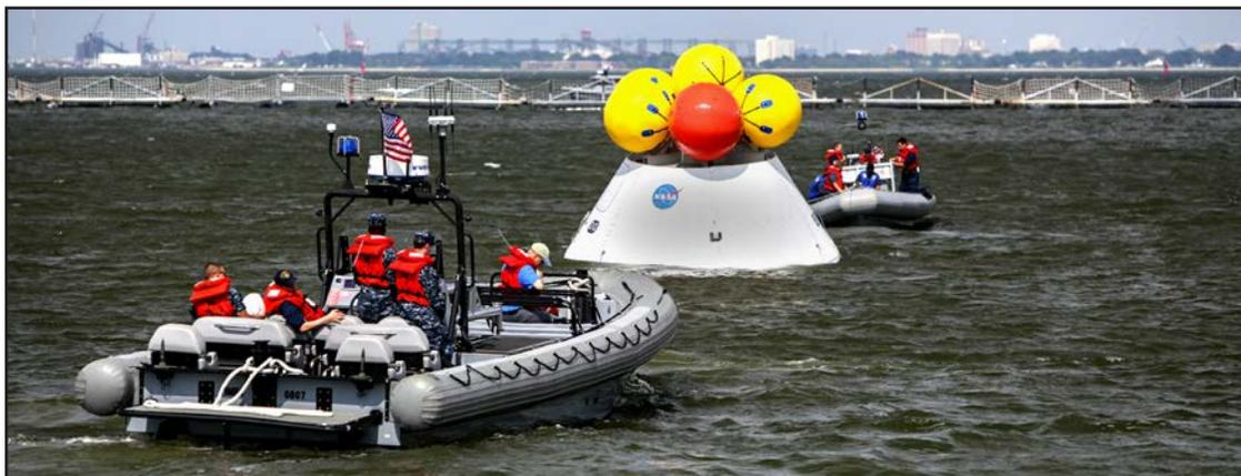
A stationary recovery test using the Orion boilerplate test article was conducted at the Naval Station Norfolk near NASA's Langley Research Center in Virginia on Aug. 15, 2013. A second test will be conducted this year in the open waters of the Pacific Ocean.
