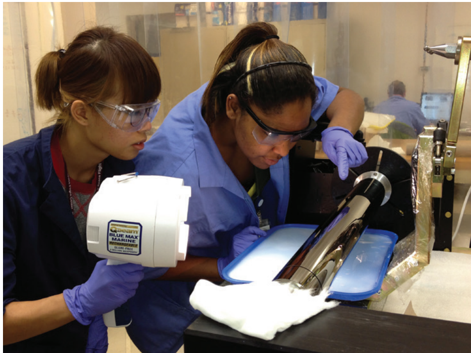
ENR fabrication enables fast, affordable production of X-ray optics for next-generation instruments.
