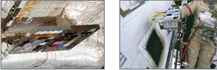
Both the **Replaceable Cassette-Container (SKK/CKK)** and Vynoslivoost Experiment Facility consist of two-flap structures and consist of a casings and spool holders that contain sample cassettes of materials of the outside surfaces of the ISS Russian Segment modules.
