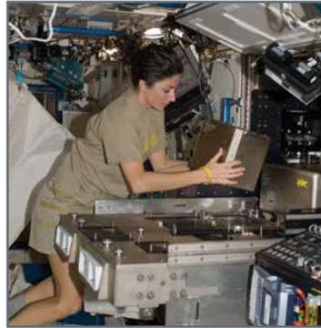
NASA astronaut Nicole Stott, Expedition 21 flight engineer, installs hardware in the FIR in the Destiny laboratory of the ISS (ISS021E011438).
