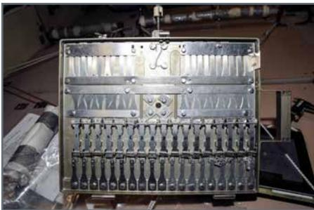
Photographic documentation taken of sample removal from Panel number 2a of the Vynoslivoost experiment in preparation for return (ISS040E109662).
