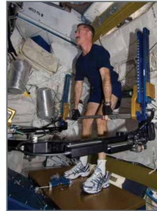
**Advanced Resistive Exercise Device (ARED)** [NASA] provides resistive exercise capabilities to crewmembers on the ISS. The **ARED** also collects data regarding the parameters (loads, repetitions, stroke, etc.) associated with crew exercise, and transmits it to the ground.
