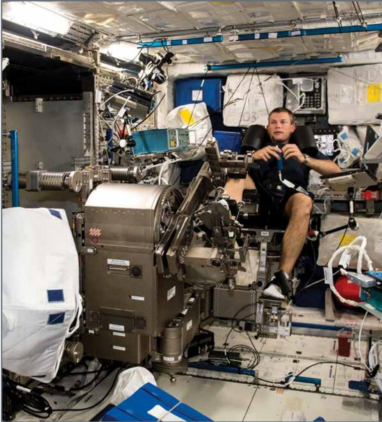
ISS crewmember Andreas Mogensen setting up the ESA MARES rack and its ankle mechanism in the Columbus module. PEMS is located to the right (ISS044E101255).
