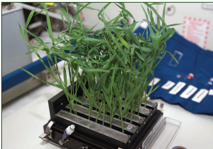
Figure 1. Wheat cv. USU Apogee grown in Biomass Production System during Photosynthesis Experiment and System Testing and Operation experiment during International Space Station Increment IV. (Source: NASA)
