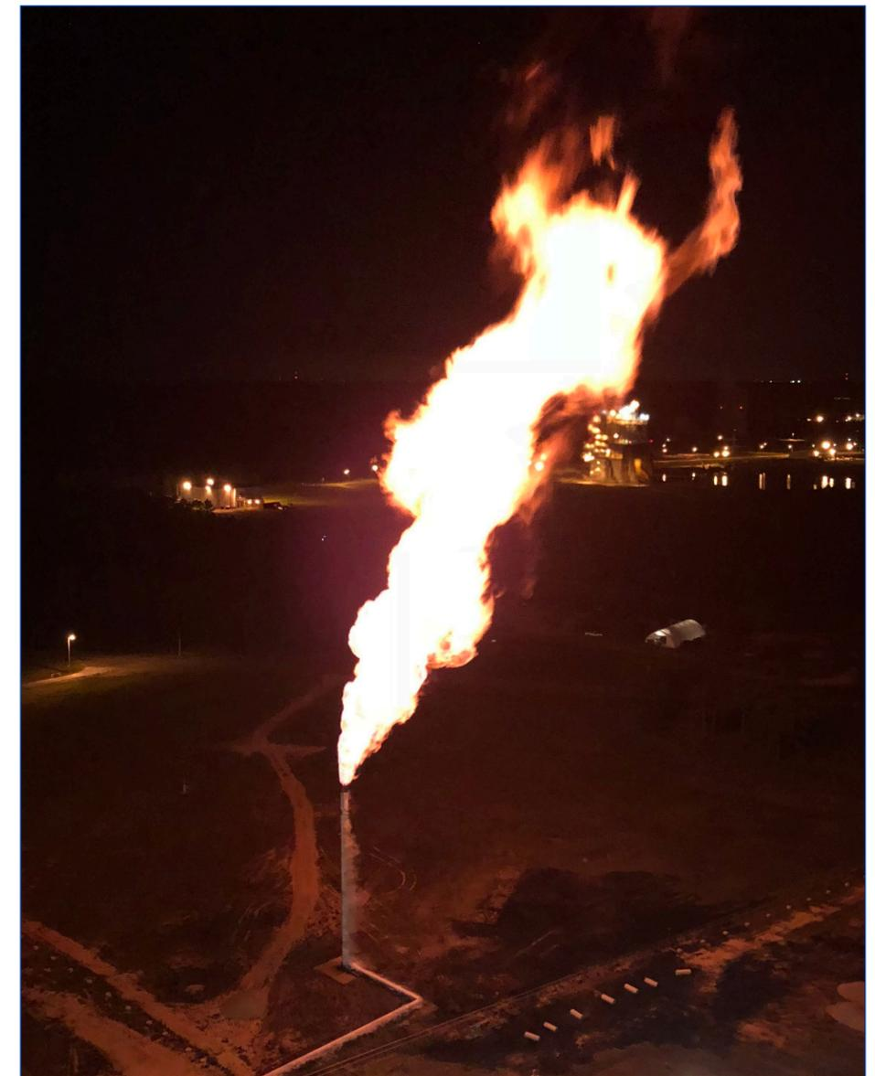
Liquid hydrogen is burned out through a flare stack at the B-2 Test Stand during a propellant cold flow test. The successful cold flow test marked a major milestone in activation of the stand for testing NASA's SLS core stage.
