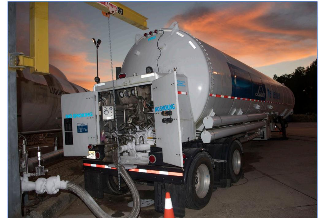
(Left photo) Heavy condensation early on the morning of Oct. 19 signals the transfer of super-cold liquid nitrogen into large vaporizers used to convert the liquid to a gaseous state at the Stennis Space Center high-pressure gas facility. Operators conducted a critical "stress test" of gas house capabilities Oct. 18-19 to demonstrate its readiness for upcoming testing of the core stage of NASA's new Space Launch System rocket.
