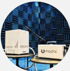
[Mochii](#) is a miniature scanning electron microscope that helps in rapid identification of particles found on the space station, many invisible to the naked eye. Such particles can cause vehicle and equipment malfunctions and threaten crew health, but currently, samples must be returned to Earth for analysis, leaving crew and vehicle at risk. Mochii also provides a powerful new analysis platform to support novel microgravity science and engineering.
