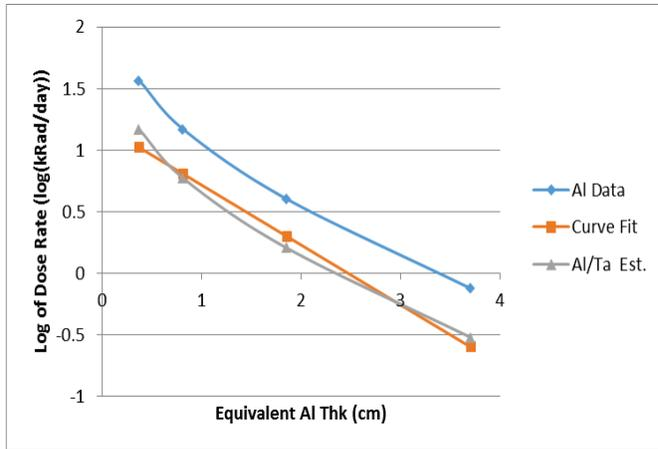
**Figure 2-6: Radiation Dose v. Shield Thickness Approximation**
