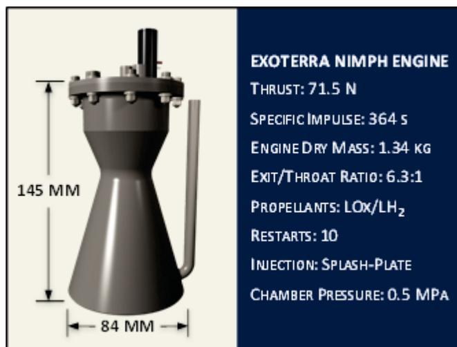
Figure 4-2: Details of the NIMPH Main Engine
