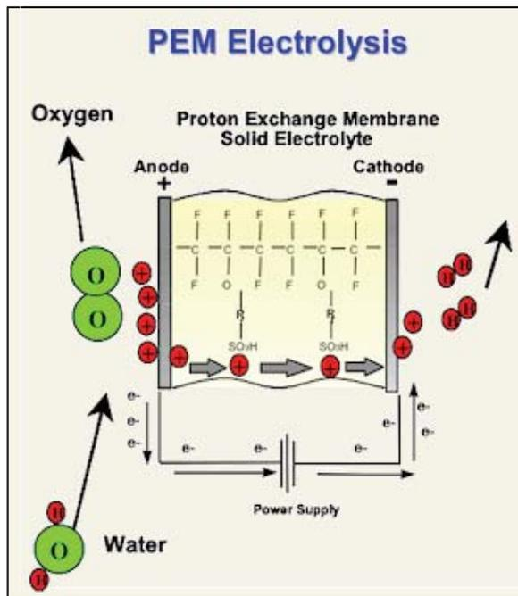
Figure 3-5: PEM Electrolysis
