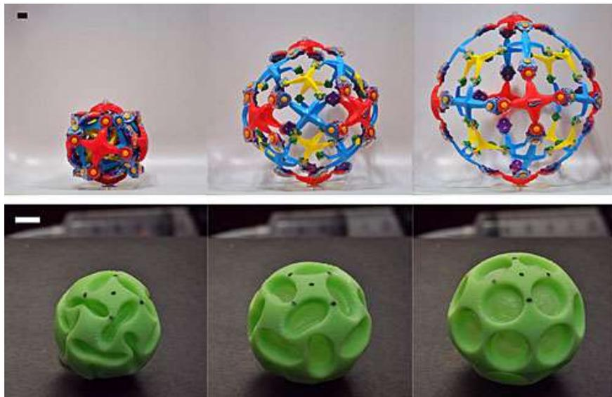
Figure 4-9: Buckliball – 3D origami like structure that collapses to 46% its original size [46].
