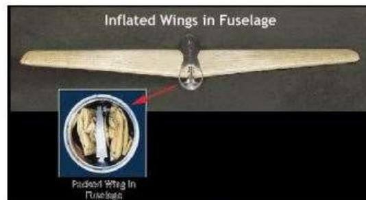
Figure 3-21: ILC Dovers multi-spar inflated wing and packed configuration [42].
