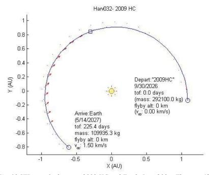
Fig. 10 STP transfer between 2009 HC and Earth.  $I_{sp} = 200 \text{ s}$ , Thrust =  $45N \otimes 1 \text{ AU}$
