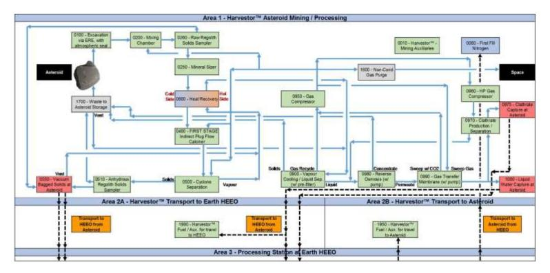
Fig. 7 Analysis of at-the-asteroid processing identified 13 major phases. The estimates for mass, power, and throughput will be greatly refined during Phase II work.
