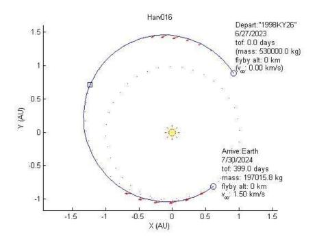
Fig. 11 STP transfer between 1998 KY26 and Earth.  $I_{sp} = 200 \text{ s}$ , Thrust = 80N @ 1 AU
