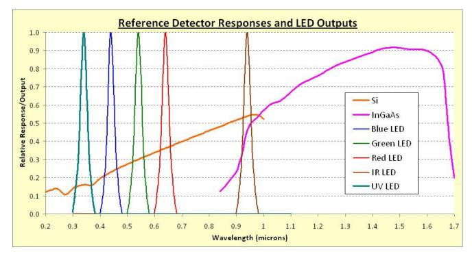
Figure 3-10: Five LED emission lines and response of Si and InGaAs monitor detectors
