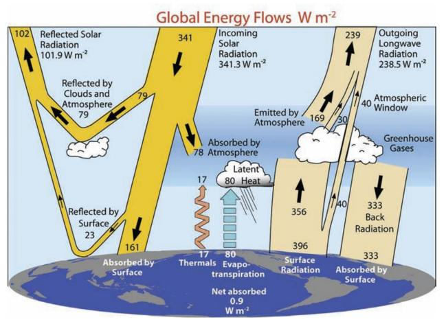
Figure 2-1: Typical radiation balance between earth, sun and space averaged over 24 hours (source: Trenberth 2010)
