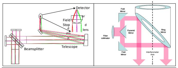
Figure 3-11: UV/VIS/NIR Optical configuration and laser metrology (only one band shown)
