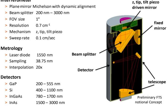
Figure 4-3: UV/VIS/NIR Fourier Transform Spectrometer Concept
