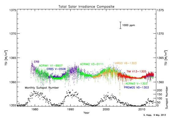
Figure 2-6 Latest composite solar irradiance record after bias removal (G. Kopp, 2013)
