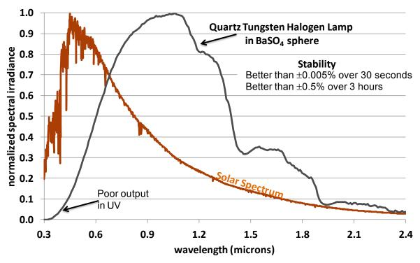
Figure 3-5: Quartz tungsten halogen bulb vs. solar spectrum
