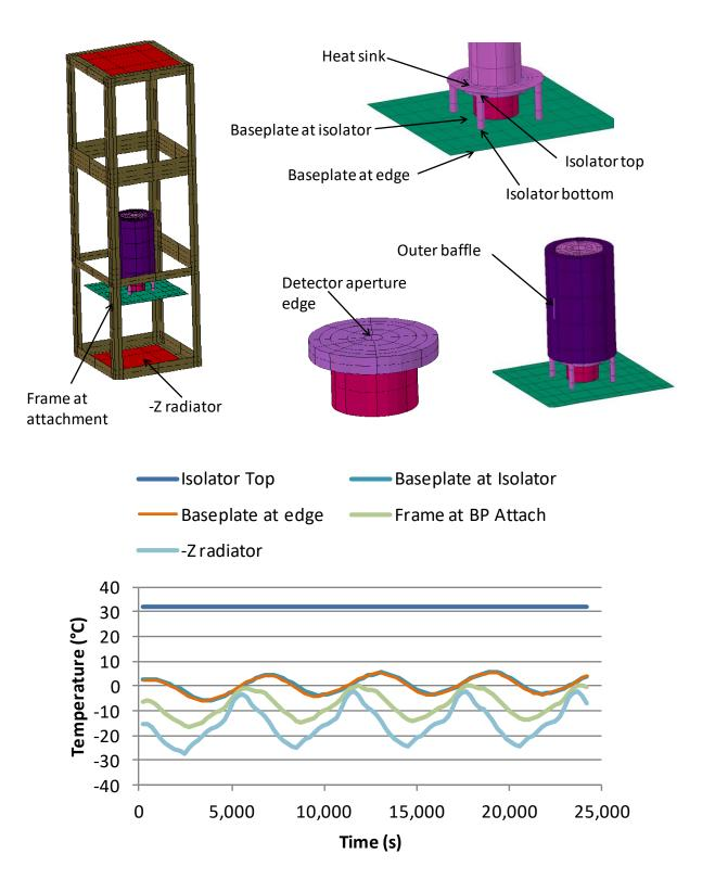
Figure 5-2: Thermal simulation of 3U Cubesat ACR & LED integrating sphere operating in an 800 km eclipse orbit
