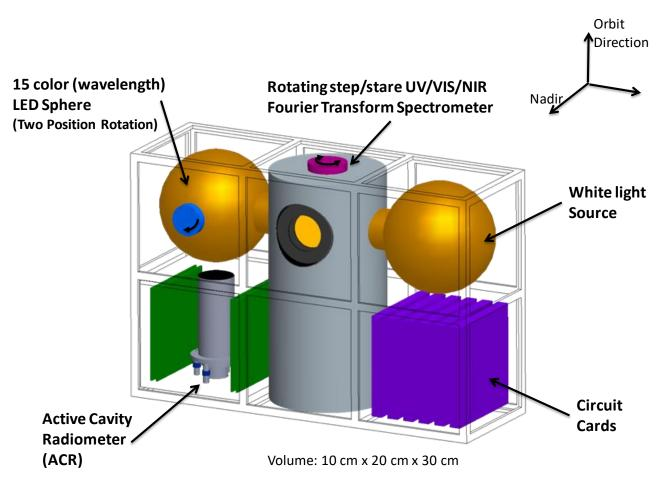
Figure 4-1: NIST-in-Space implemented as a Cross-track Earth scanner
