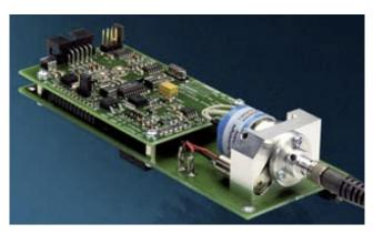
Figure 3-6: Commercial deuterium with quartz tungsten halogen lamp & fiber optic
