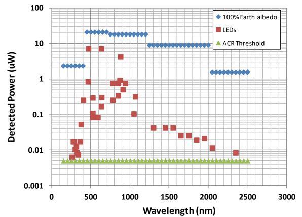
Figure 3-9: Total power detected by FTS instrument having 1° FOV and 2.5 cm aperture when viewing 100% earth albedo scene (blue) or when viewing LED driven integrating sphere (red). Note that commercially available LED chips used in this example are ~100x underpowered
