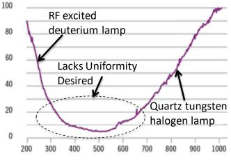
Figure 3-7: Deuterium & quartz tungsten halogen lamp spectrum
