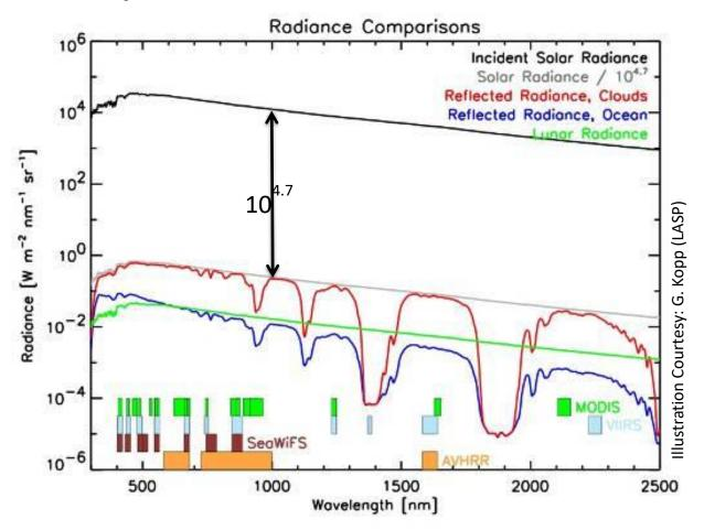
Figure 2-7: Solar radiance and earth reflected radiance differ enormously and measuring both of these accurately is very difficult (Illustration courtesy G. Kopp, LASP)
