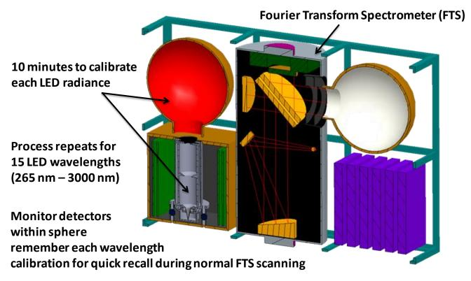
Figure 4-2: FTS scans earth and white light source while LED Sphere undergoes NIST traceable calibration by ACR
