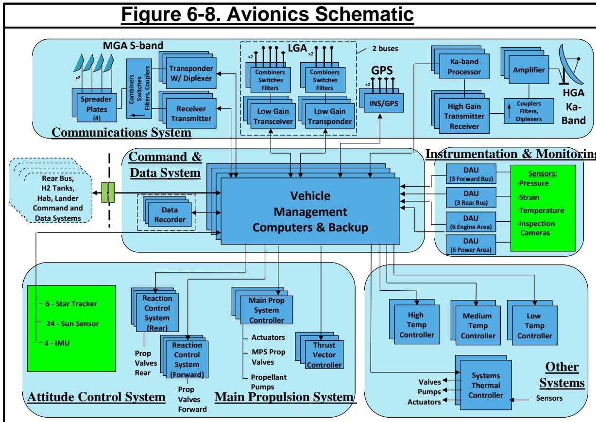
The vehicle would be in control of the flight of the stack independent of payload elements, particularly the Habitat, landers, and payloads. The Habitat would have command override capability. All elements would provide health and status instrumentation to the AFFRE vehicle.
