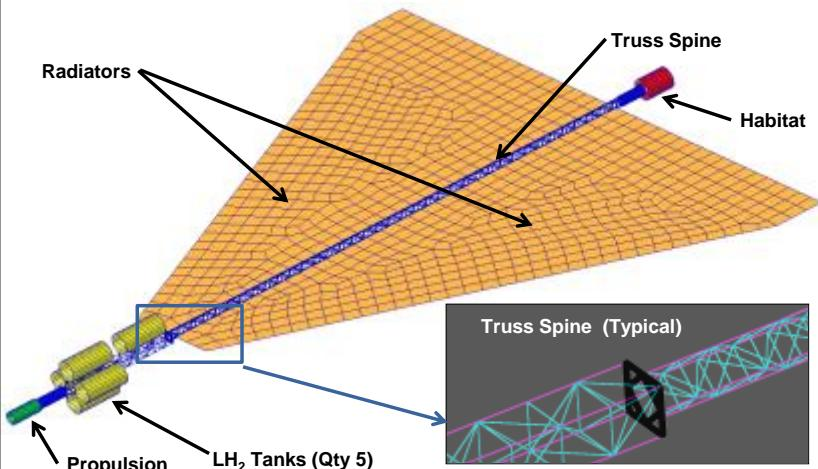
diameter and wall thickness for simplicity of analysis. The Truss Spine structure was developed using ProE CAD models.
