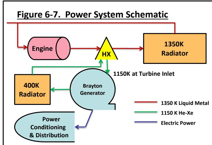
AFFRE heats liquid metal to transport the heat to the 1350K high temperature radiators. A heat exchanger is used to heat He-Xe gas to power the Brayton engine. The Brayton generator converts the thermal power to electricity and delivers He-Xe at 400K to the low temperature radiators. The power produced is managed by the PMAD system. Although three Brayton units are required, five are carried for fault tolerance.
