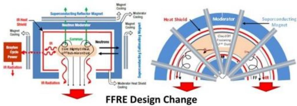
and a large enough hole to enable the magnetics to direct the fission fragments out of the reactor.
