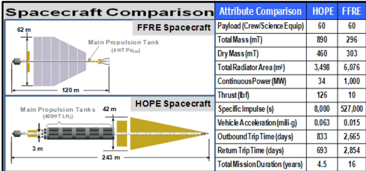
cruise liner. Further, the HOPE ship needs as much liquid hydrogen as resides in three SLS core stages. This hydrogen would have to be maintained in a cryogenic condition throughout the mission, a formidable task. These immense hydrogen tanks would be shed as the propellant is consumed during each mission burn. Consequently for another mission, at least five Heavy Lift flights would be needed just for replenishment of the needed hydrogen and for new tanks.
