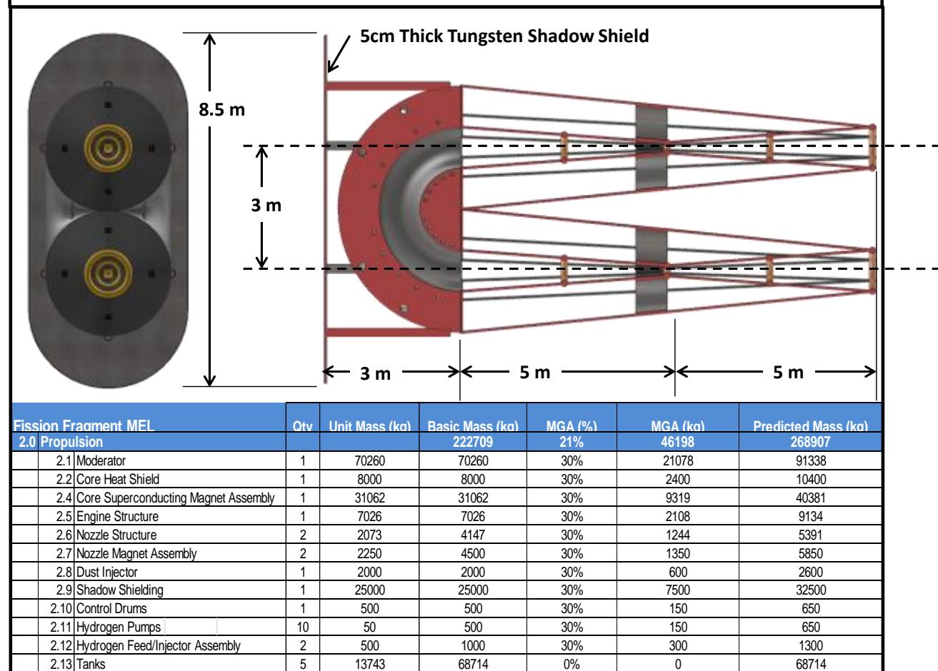
is constructed using carbon-carbon tubes to allow for the reflected IR radiation to escape with minimal impact to the nozzle assembly. The structure supports four magnetic beryllium rings of varying sizes. The nozzle converges to a 20 cm nozzle diameter. The four magnetic rings help to direct the fission
