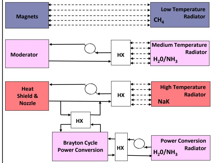
medium temperature radiator system for the moderator, a high temperature radiator to cool the moderator heat shield and nozzle, and a second medium temperature radiator for the Brayton power conversion system for heat rejection.
