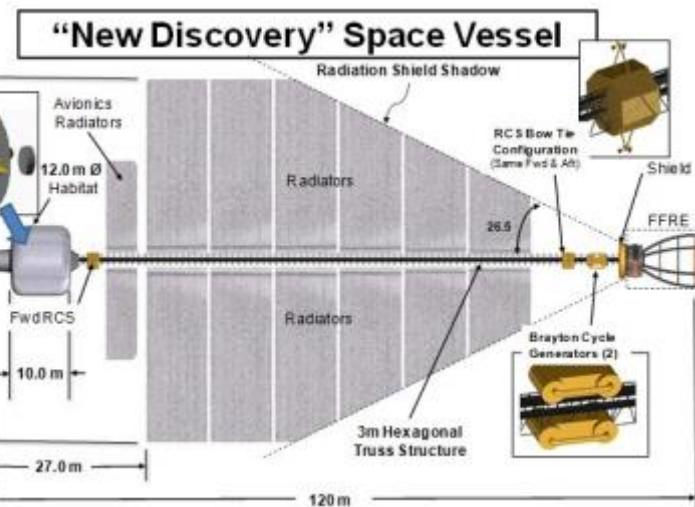
The physical comparison, shown in the figure on the next page, reveals the significant impact the opposing engine technologies have on vehicle configuration. The FFRE, with a specific impulse so great that it consumes an insignificant propellant quantity, shortens “New Discovery” to a vessel of about ISS dimensions whereas the MPD engines make the HOPE vehicle the size of a
