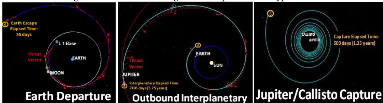
To simplify the analysis, the trajectory was segmented based on which was the “primary gravitational attractor”: Earth, Sun, or Jupiter, as shown in the above figures. Once the Earth escape velocity was achieved at waypoint “A” for example, the trajectory computation was shifted from an Earth-centered system to a Sun-centered one.
