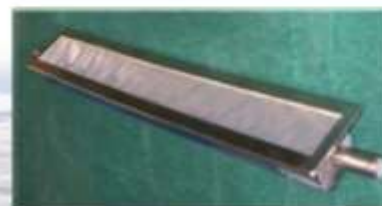
Screen channel capillary LAD
