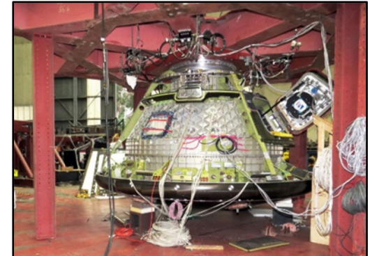
Fixed Tunnel Test: Unit & Ascent Loads
