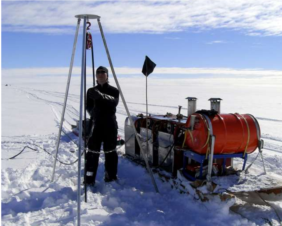
NSF Ice Drilling Development Office (IDDO) portable hot water drill. Image from: http://icedrill.org/equipment/portable-hot-water-drills.shtml
