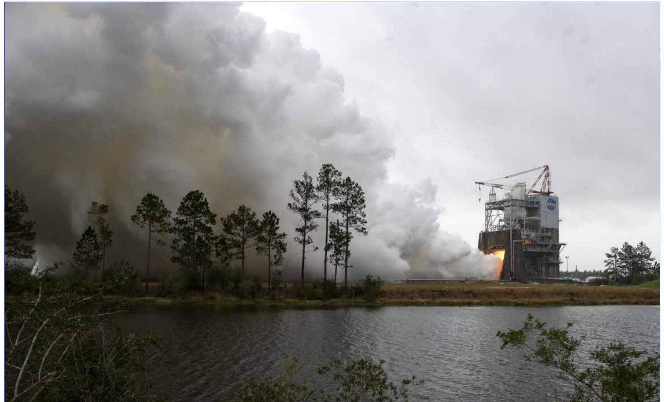
NASA engineers conduct a successful test firing of RS-25 rocket engine No. 2059 on the A-1 Test Stand at Stennis. The hot fire marks the first test of an RS-25 flight
