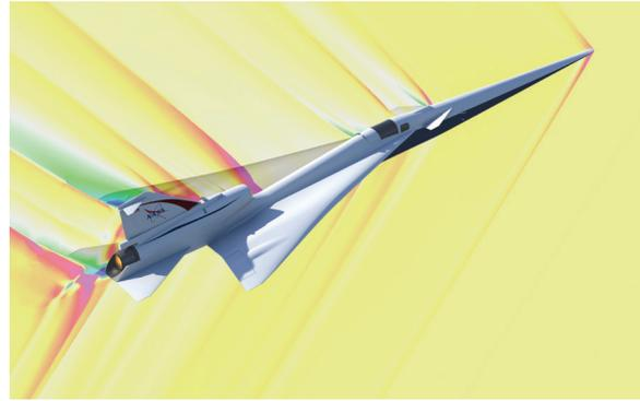
Computer simulation showing how shockwaves move away from the X-59 as it flies faster than sound. The pattern is different from the way shockwaves from a conventional supersonic aircraft come together to produce a sonic boom. Instead, the X-59 will produce a quieter sonic thump.
