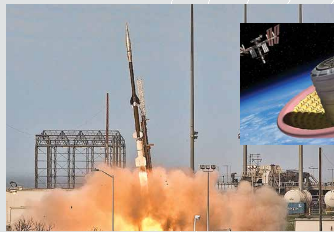
IRVE-3 launches aboard a Black Brant rocket at Wallops Flight Facility carrying an experimental inflatable heat shield.
