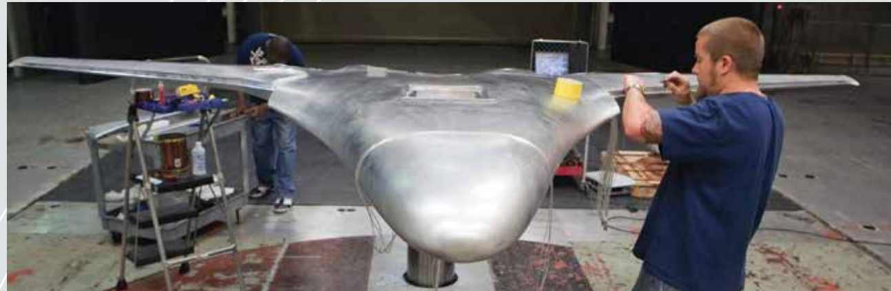
A technician works on a hybrid wing body model in a Langley wind tunnel.
