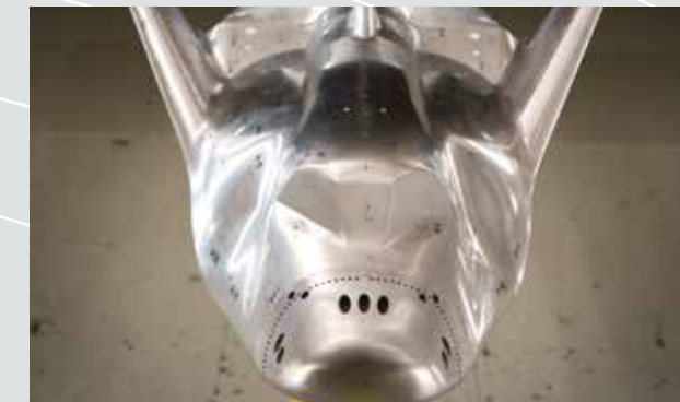
A Dream Chaser spacecraft model in a Langley wind tunnel.
