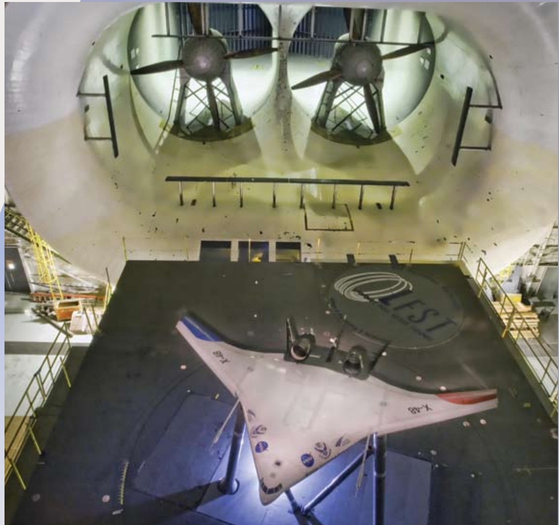
(Above) The X-48C 8.5% scale blended wing-body flight test aircraft undergoes evaluation in the final test in Langley's historic 30 x 60- Foot Wind Tunnel. The tunnel has evaluated nearly every type of aircraft since it was constructed in 1930.
