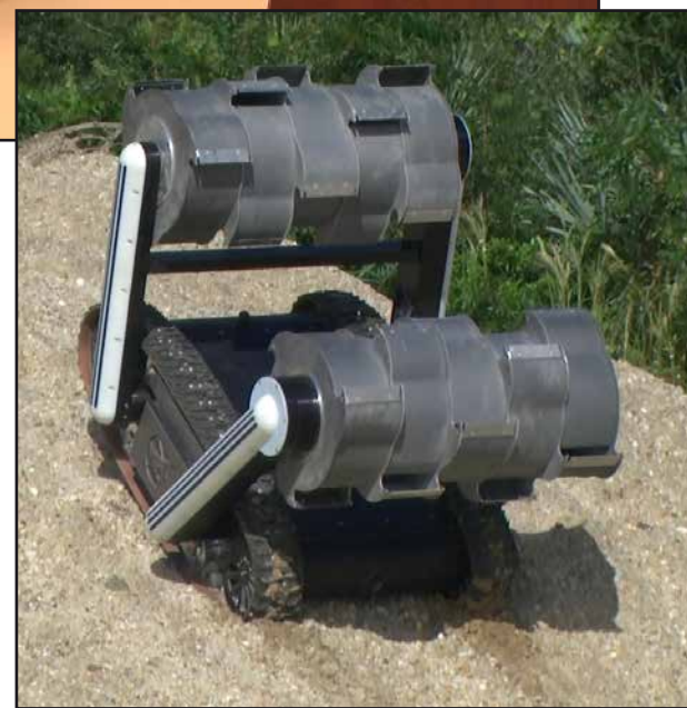
NASA's prototype Regolith Advanced Surface Systems Operations Robot (RASSOR) will be incorporated into the "swarmies" tests to see how well the software translates to different robotic vehicles. RASSOR is a concept robotic vehicle evaluating designs for a future craft that could work on another world. Photo credit: NASA
