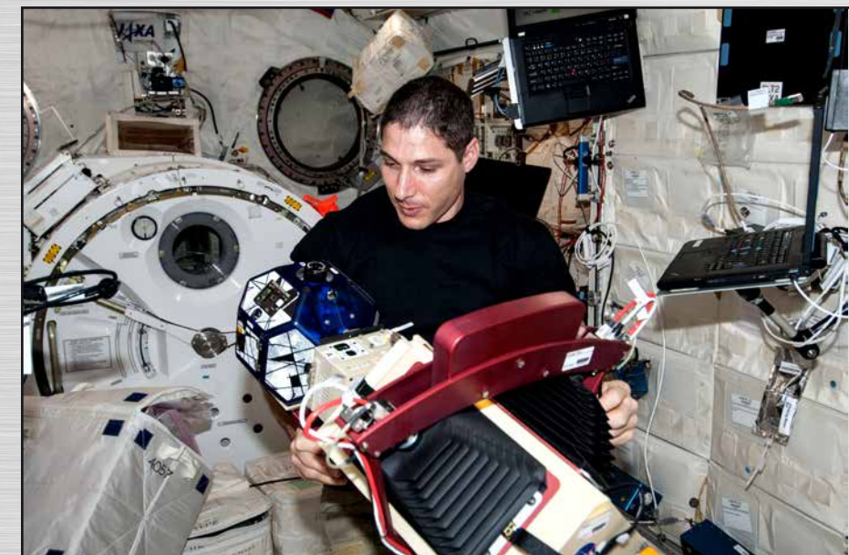
Aboard the International Space Station on Jan. 22, 2014, Expedition 38 flight engineer Mike Hopkins works with the SLOSH experiment developed by engineers at Kennedy. The device is now being used on the space station to better understand how liquid propellants perform in a reduced-gravity environment. Photo Credit: NASA
