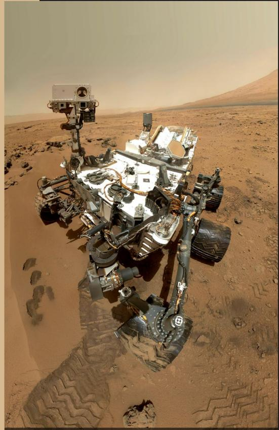
NASA's Curiosity rover used the Mars Hand Lens Imager to capture this set of 55 high-resolution images, which were stitched together to create this selfie. Taken on Oct. 31, 2012, it shows the rover at the site where the mission's first scoop sampling took place. Four scoop scars can be seen in the regolith in front of the rover. The base of Gale Crater's 3-mile-high sedimentary mountain, Mount Sharp, rises in the right side of the frame Image credit: NASA/Jet Propulsion Laboratory-Caltech
