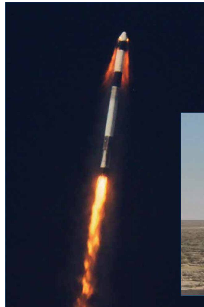
Left: The uncrewed SpaceX Crew Dragon capsule separates from the company's Falcon 9 rocket during an in-flight abort test following liftoff from Kennedy Space Center's Launch Complex 39A on Jan. 19, 2020. Photo credit: SpaceX
