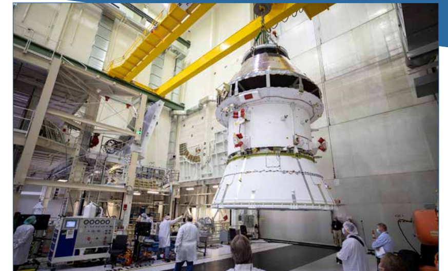
The Artemis I Orion spacecraft, with its spacecraft adapter cone attached, is moved by crane along the high bay inside Kennedy's Neil Armstrong Operations and Checkout Building on Aug. 20, 2020.
