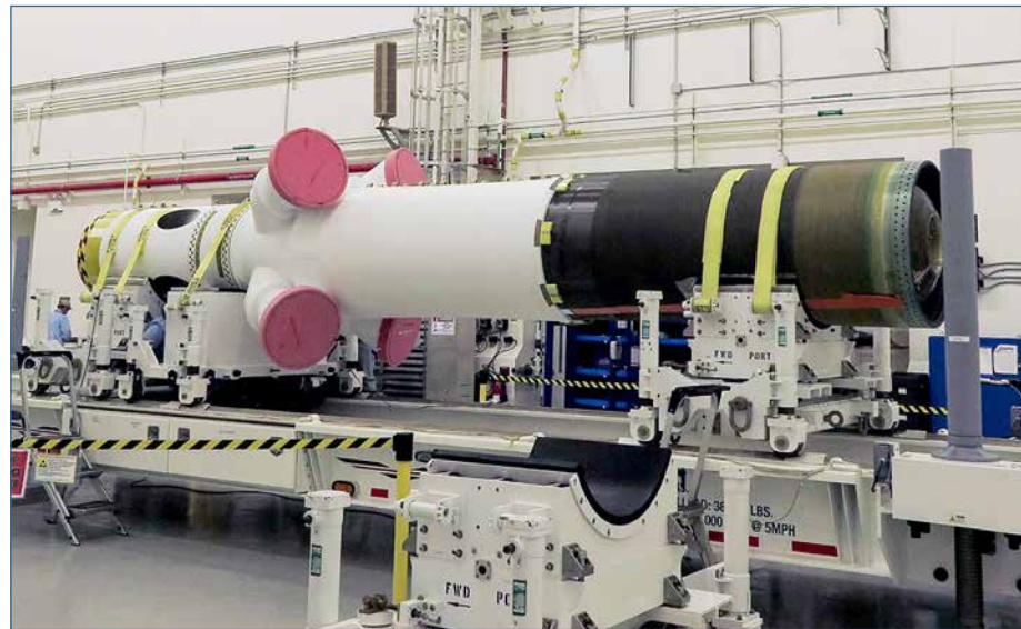
The launch abort motor is integrated with the jettison motor for Orion's launch abort system for Artemis II inside Kennedy's Launch Abort System Facility on April 15, 2020. Photo credit: Lockheed Martin
