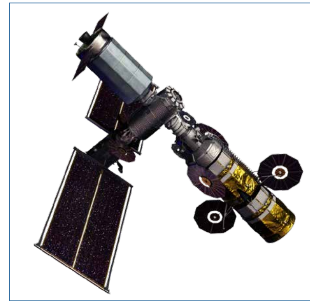
NASA's Phase 1 Gateway includes a Power and Propulsion Element combined with a Habitation and Logistics Outpost and logistic supply.
