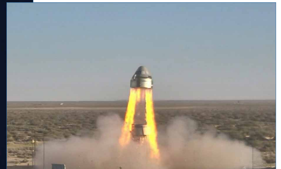
Below: The Boeing CST-100 Starliner's four launch abort engines and several orbital maneuvering and attitude control thrusters ignite in the company's uncrewed Pad Abort Test on Nov. 4, 2019, from Launch Complex 32 on White Sands Missile Range in New Mexico.
