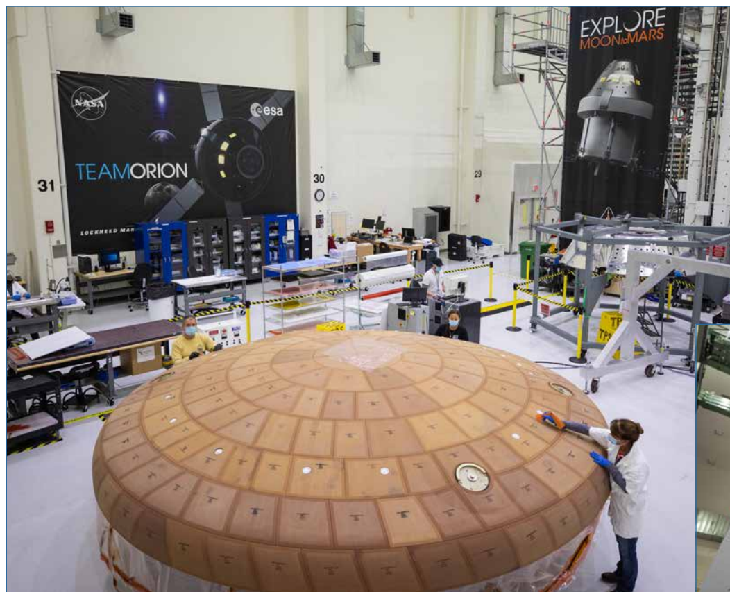
Technicians with ASRC Federal inspect AVCOAT block bonding on the Artemis II heat shield inside Kennedy's Neil Armstrong Operations and Checkout Building on July 2, 2020.
