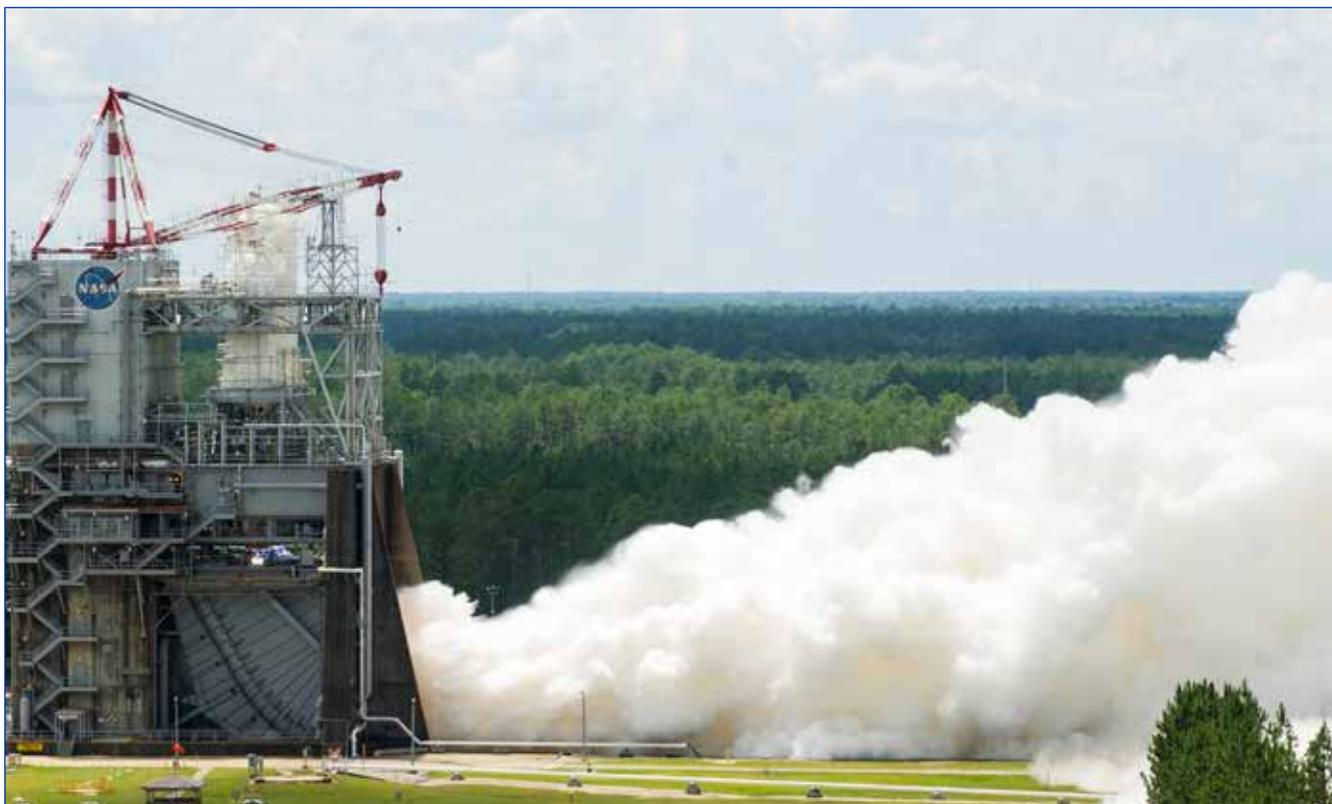
An RS-25 engine fired up for 500 seconds June 11 at Stennis Space Center. It was the third firing of an RS-25 development engine on the A-1 test stand at Stennis, with four more tests planned for the current development engine.
