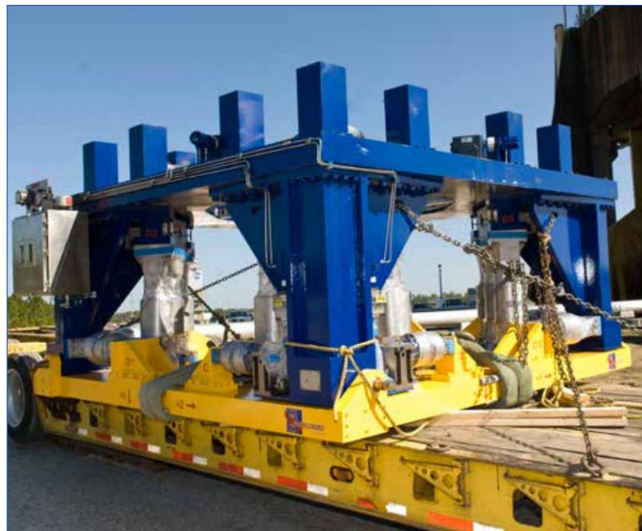
A state-of-the-art thrust measurement system arrives at the A-1 Test Stand for installation in 2010. The system is a precisely calibrated component used to collect thrust data during a rocket engine test.
