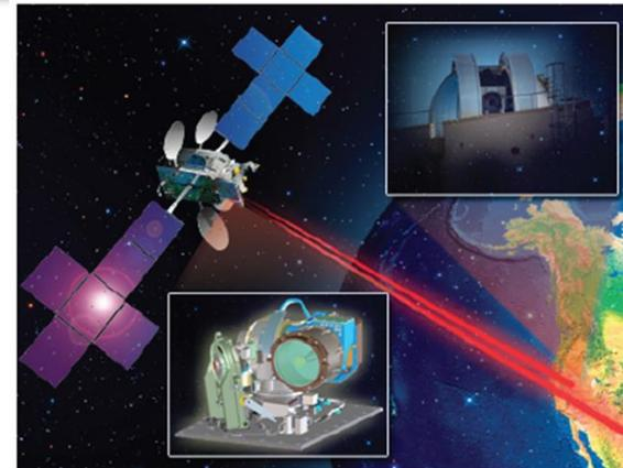
LCRD is a hosted payload on an SSL commercial telecom satellite
