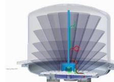
Radio Frequency Mass Gauge (RFGM) for Robotics Refueling Mission 3 (RRM3)
