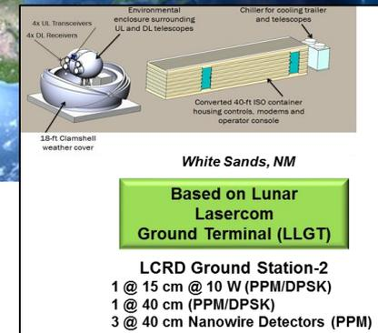
KDP-A/B architecture - LCRD on SSL commercial telecom satellite, with 2 ground stations (GS-1 at OCTL and GS-2 at White Sands)
