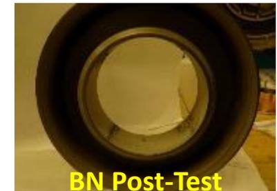
Post-test BN discharge chamber shows carbon deposition consistent with magnetically shielded operation
