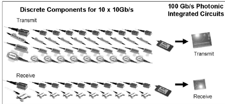
...into the optical equivalent of a micro-electronics “integrated circuit”
