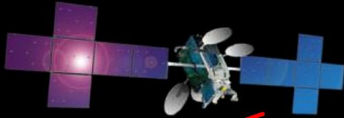
Currently Funded: Laser Communications Relay Demonstration (LCRD) in GEO With 2 "Traditional" Modems at 2.88 Gbps
