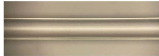
Figure 3-3. ZBLAN fiber from Spool 15 (LVF preform)
