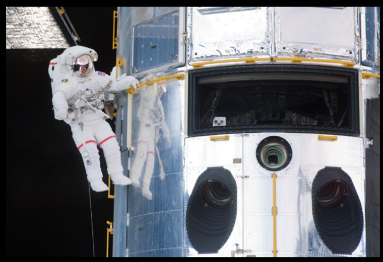
Astronaut John Grunsfeld performs work on the *Hubble Space Telescope* during the first of five spacewalks conducted on the last servicing mission in 2009. Credit: NASA
