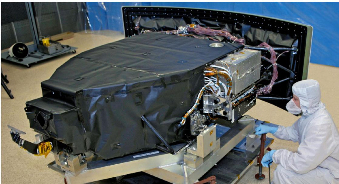
NIR instrument that used a cryogenic cooler that last operated in 2008. Compared to NICMOS, WFC3 has six times the NIR field of view and 16 times as many pixels.
