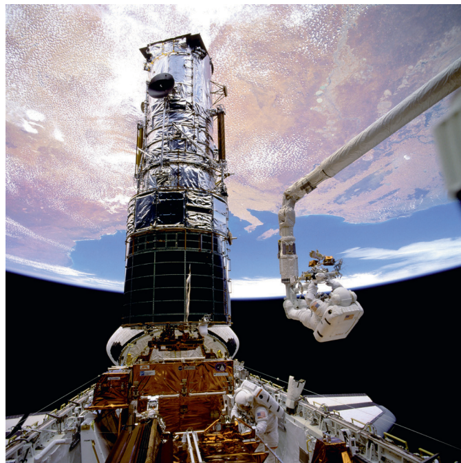
Astronauts F. Story Musgrave (anchored on the end of the Remote Manipulator System arm) and Jeffrey A. Hoffman (bottom of frame) work on Hubble during the first servicing mission in December 1993.
