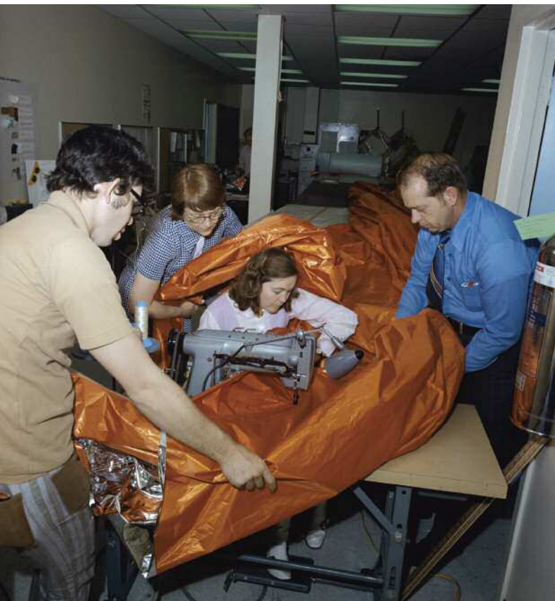
MSC employees help a seamstress feed material through a sewing machine to create the three-layered sunshade for use as a parasol to protect the Skylab space station from excessive heat after it was damaged during launch.
