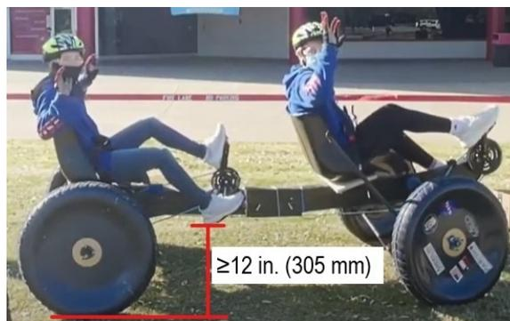
*Figure 1: Vehicle Height Requirement*
