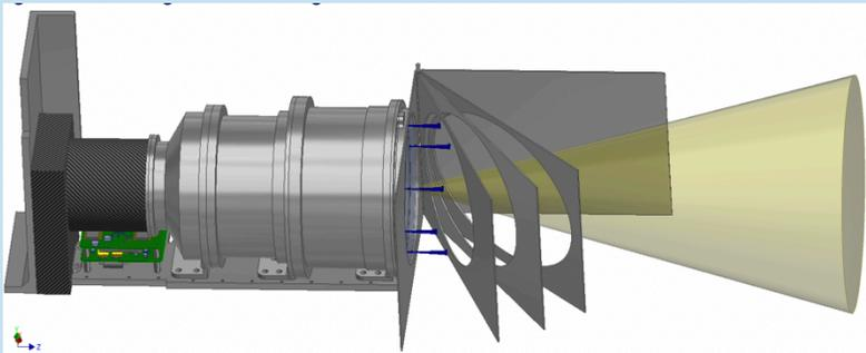
13 cm, 6 element refractive telescopes • **High-efficiency delta-doped CCD detectors (JPL)** • High-transmission GdF<sub>3</sub> anti-reflection coatings (GSFC) • Deployable straylight baffles
