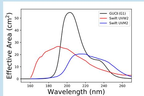
The high-efficiency delta-doped CCDs and high-transmission anti-reflection coatings enable GUCI to achieve a larger effective area than *Swift*-UVOT, despite a much smaller aperture (13 vs 30 cm)
