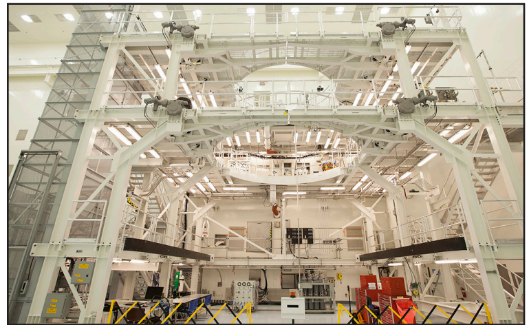
The Orion service platform will be used for offline processing and fueling of the Orion spacecraft and service module stack before launch. Modifications now are complete with validations and testing underway. Photo credit: NASA/Ben Smegelsky
