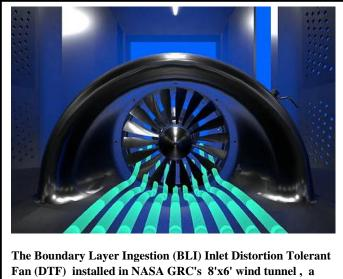
Fine Boundary Layer ingestion (BL1) milet Distortion Tolerant Fan (DTF) installed in NASA GRC's 8'x6' wind tunnel, a new capability to investigate fuel burn reduction potential by embedding an aircraft's engine at the rear of an aircraft compared to an under the wing conventional configuration.
