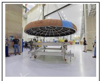
October 23, 2017 Orion heat shield for EM-1 moves toward the thermal chamber in Neil Armstrong Operations and Checkout building at NASA's KSC in Florida. It will undergo a thermal cycle test to verify acceptable workmanship and material quality.
