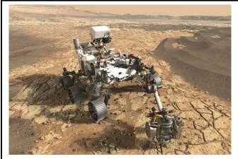
Mars 2020 will re-use the basic engineering of NASA's Mars Science Laboratory to send a different rover to Mars, with new objectives and instruments, launching in 2020. The rover will carry seven instruments to conduct its science and exploration technology investigations including two contributed by international partners and one to demonstrate a critical technology for future human exploration.
