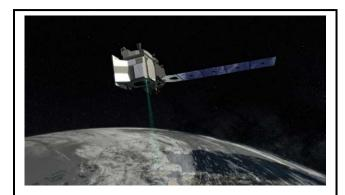
ICESat-2 will use a multi-beam micropulse laser altimeter to measure the topography of the Greenland and Antarctic ice sheets as well as the thickness of Arctic and Antarctic sea ice. The satellite LIDAR also will measure vegetation canopy heights and support other NASA environmental monitoring missions. By discovering the anatomy of ice loss, researchers may be able to forecast how the ice sheets will melt in the future and what impact this will have on sea-levels.
