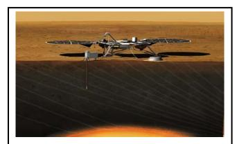
Scientists have determined the deep structure of only one planet: Earth. To obtain vital clues to how Mars formed, InSight will deploy a German-built drill nicknamed "The Mole" to pound 16 feet into the Martian crust for thermal measurements, and a sensitive French-built seismometer to detect "Marsquakes." Through these and other instruments, scientists will be able to deduce the deep structure of Mars, which currently is a mystery.
