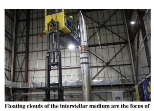
the NASA-funded CHESS sounding rocket mission, which investigates the earliest stages of star formation. Here, the CHESS payload joins with the sounding rocket before launch. CHESS launched on June 27, 2017, at 1:10 a.m. EDT from the White Sands Missile Range in New Mexico.
