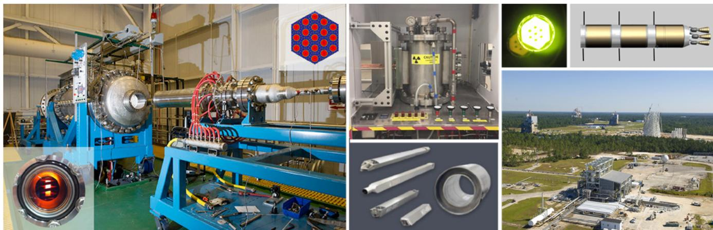
*Above left: NTREES test facility; Insets: top right, core design; lower left, prototype testing. Top center: CFEET tester, lower center: fuel rod samples. Above right: CFEET element test, conceptual craft; lower right, testing facilities at Stennis Space Center*
