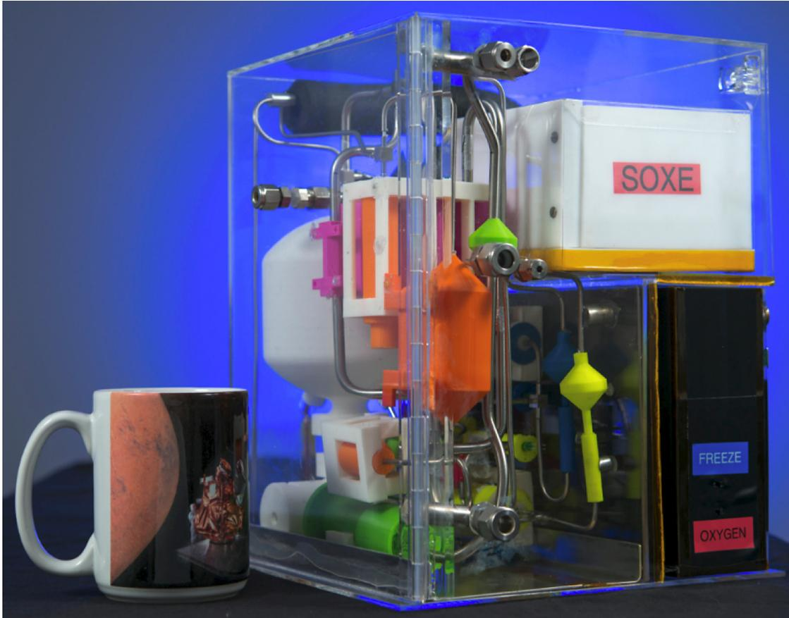
3D-printed model of the preliminary MOXIE payload. Image credit: NASA's Jet Propulsion Laboratory.
